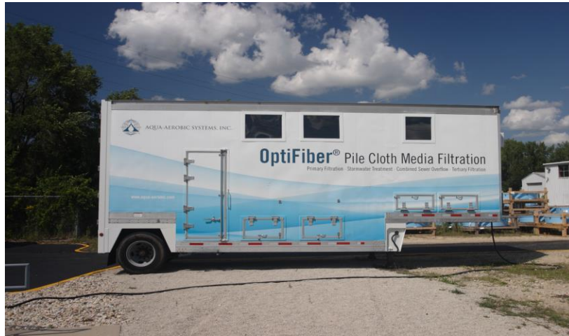
Figure 11: Primary Filtration and Wet Weather Pilot System
