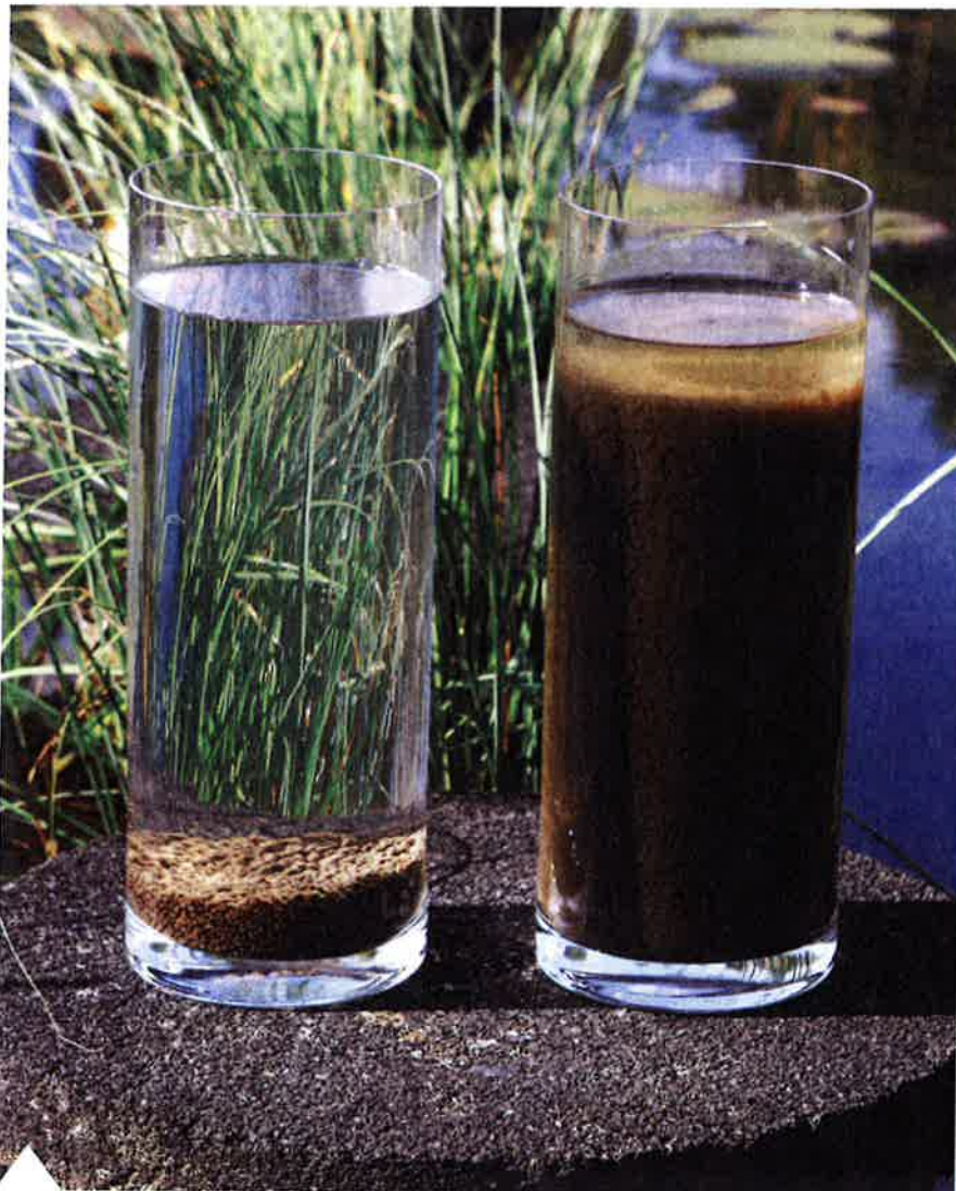
Nereda aerobic granules (left) compared to traditional activated sludge (right).
