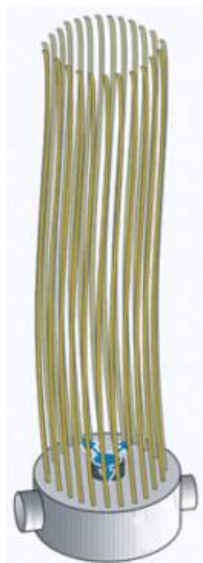
Figure 14: MBR Membrane Fiber Bundle
