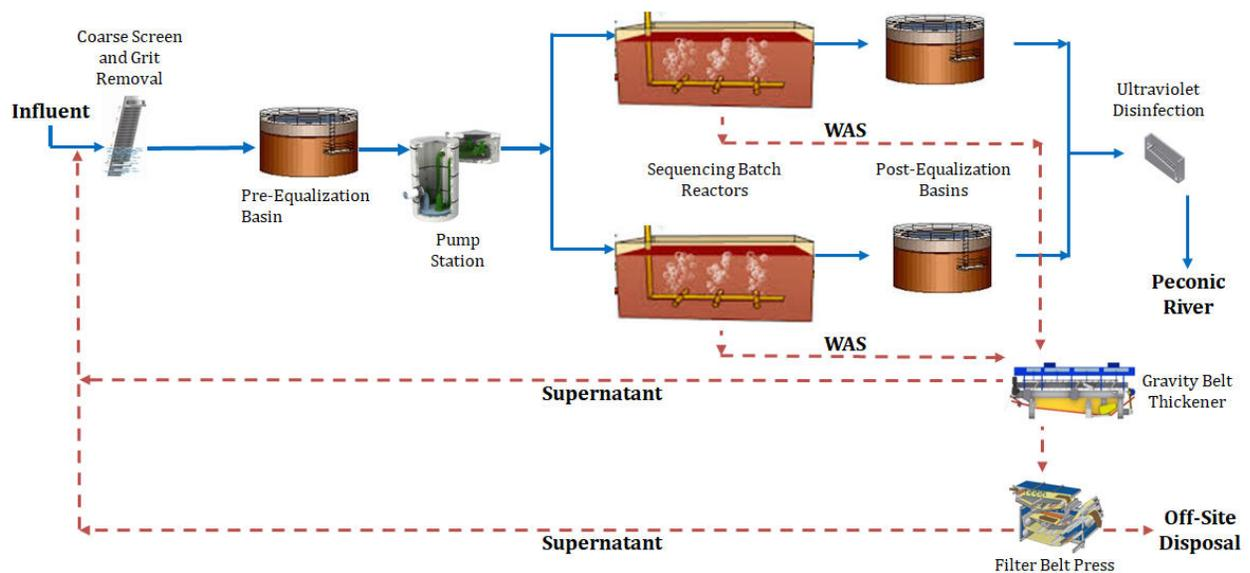
Figure 4: SBR System as Installed in 2000
