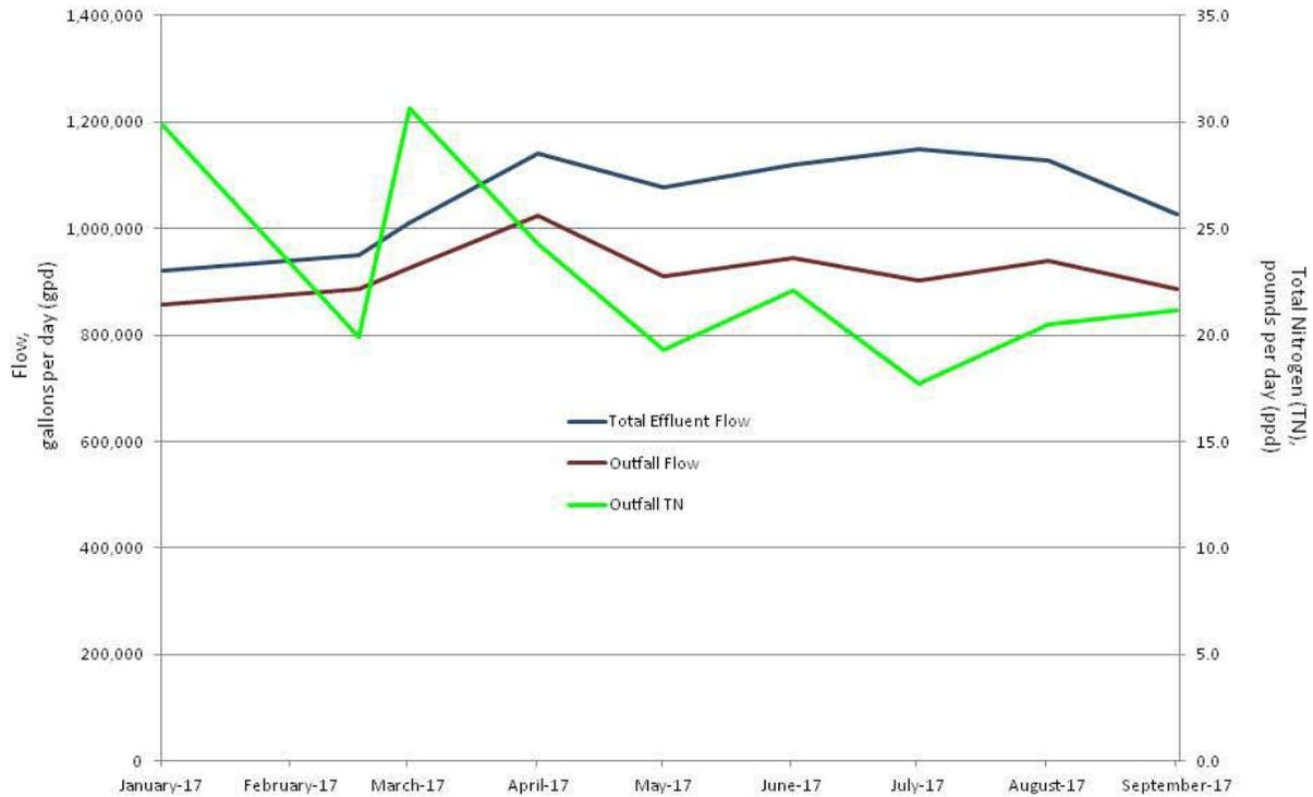
Figure 7: Flows and Total Nitrogen (TN) TMDLs
