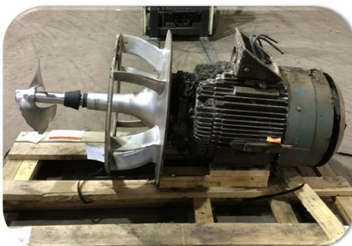
Aqua-Jet® Aerator Power Section Prior to Rebuild
