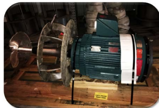
"Good As New" Aqua-Jet® Aerator Power Section
