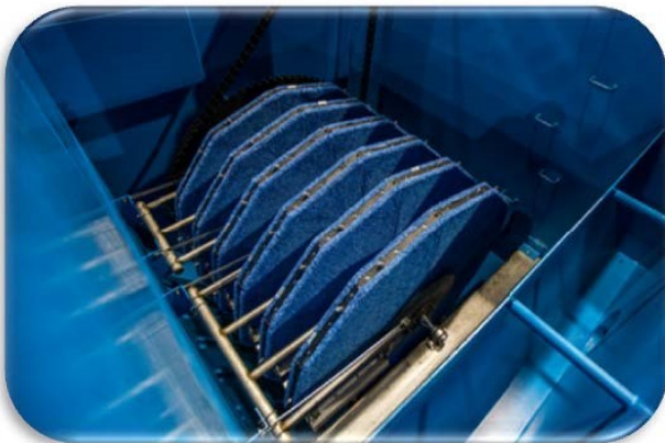
Internal components are assembled from 304 SS
