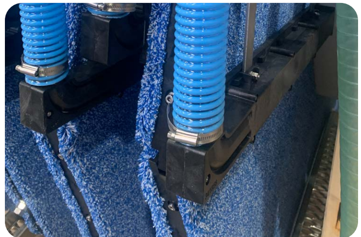
Stacked backwash shoes allowing for tighter disk spacing
