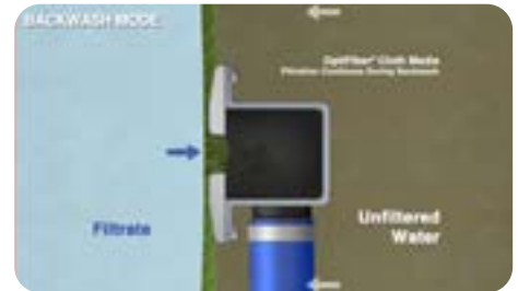
Engineered backwash shoe is optimized for complete removal of solids from the media.
