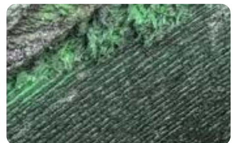
Pile cloth media in its conditioned state with the OptiComb® Backwash System
