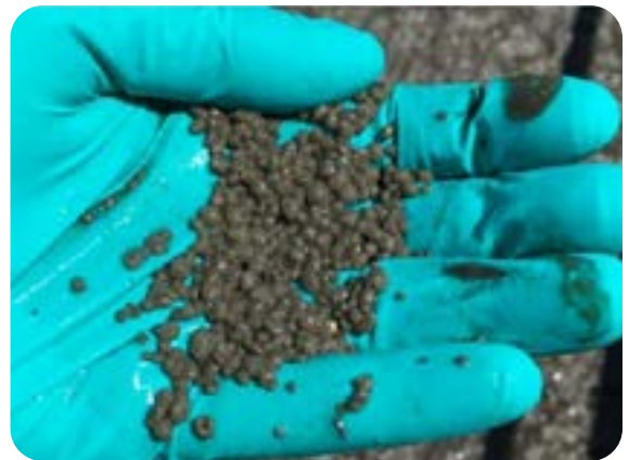
Granule sample following sieve testing at the AquaNereda® demonstration facility, Rockford, IL
