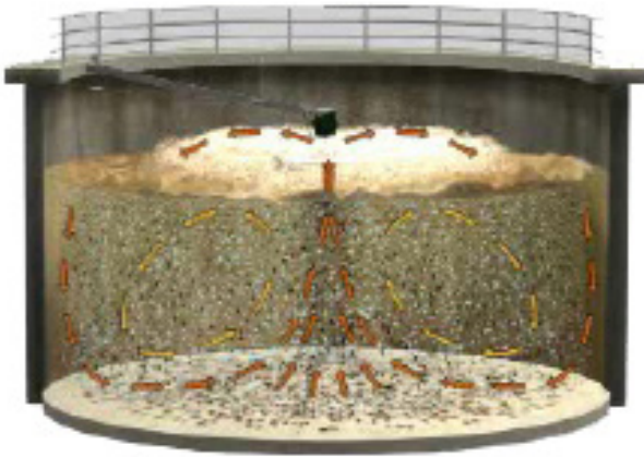
Illustration of the Aqua-Jet® Spray Pattern
