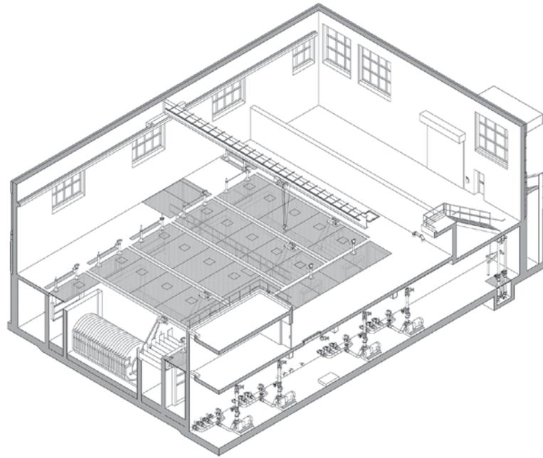
directed to UV disinfection. Designing the tertiary filter system on peak day (2.0 peak factor) rather than peak instantaneous flow (PIF) (3.5 peak factor) allowed for a reduction in the number of filters and the overall building size without impacting the plant's ability to achieve compliance objectives.
